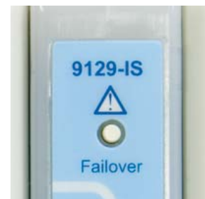
Figure 5.1 SAM failover switch button
