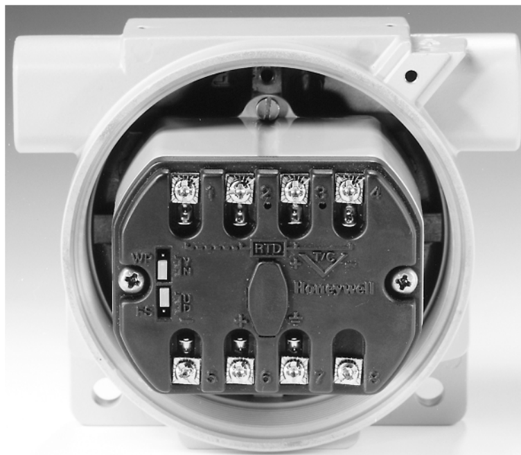
Figure 1 – STT350 Transmitter in Field Mount Housing.
