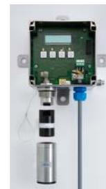
Inserting the sensor module converts the gas -neutral sensor head into a gas specific gas detector. The stainless steel cartridge can stay in place, even if the sensor is not yet built in and thus protects the interior sensor head from dust and rain.
