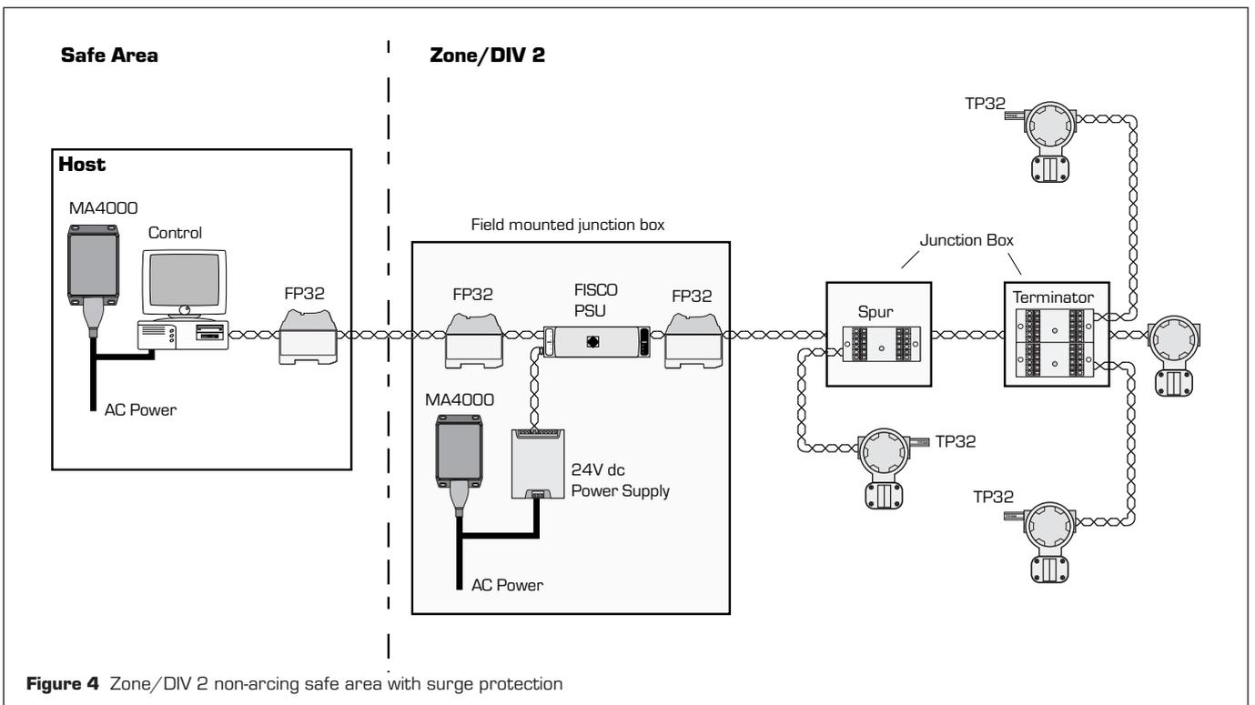
**Figure 4** Zone/DIV 2 non-arcing safe area with surge protection
