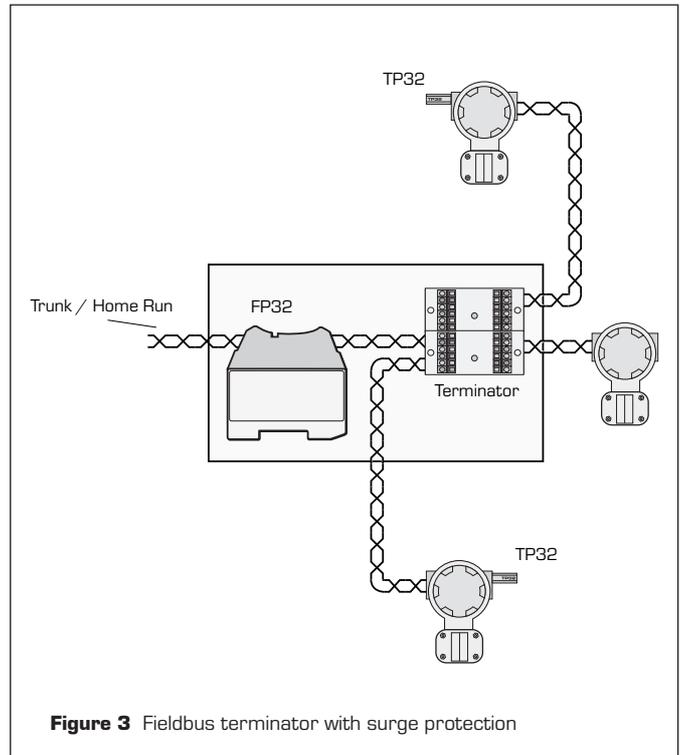
**Figure 3** Fieldbus terminator with surge protection
