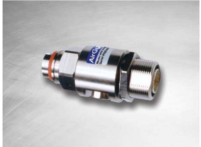
**The RGT Series** of surge protection devices prevents surges and transient overvoltages conducted through coax cables. These surge protectors employ gas tube capsules that are easily replaceable ensuring a lifetime of protection.
