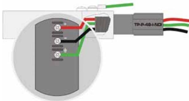
Figure 2 Connection detail for a typical process transmitter
