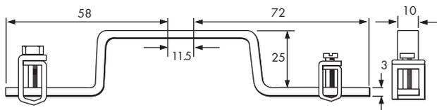
**EBB7 earth busbar** – 1 metre lengths. Mounts up to 64 barriers.
