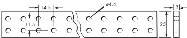
**IMB7 insulating mounting block** mounts on a flat surface or top hat rail (to EN 50 022 – 35 x 7.5; BS 5584; 35 x 27 x 7.3 DIN 46277) or G-profile rail (to EN 50 035 – G32; BS 5825; 32 DIN 46277). Recommended maximum number of barriers between blocks is 25.
