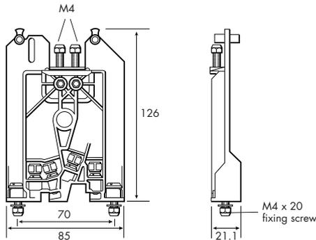
**SMB7 insulating mounting block** mounts on a flat surface and provides minimum overall installation height. Recommended maximum number of barriers between blocks is 25.
