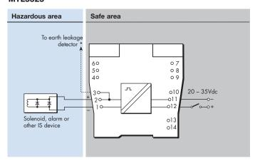
\* Signal plug HAZ1-3 is required for access to this function
